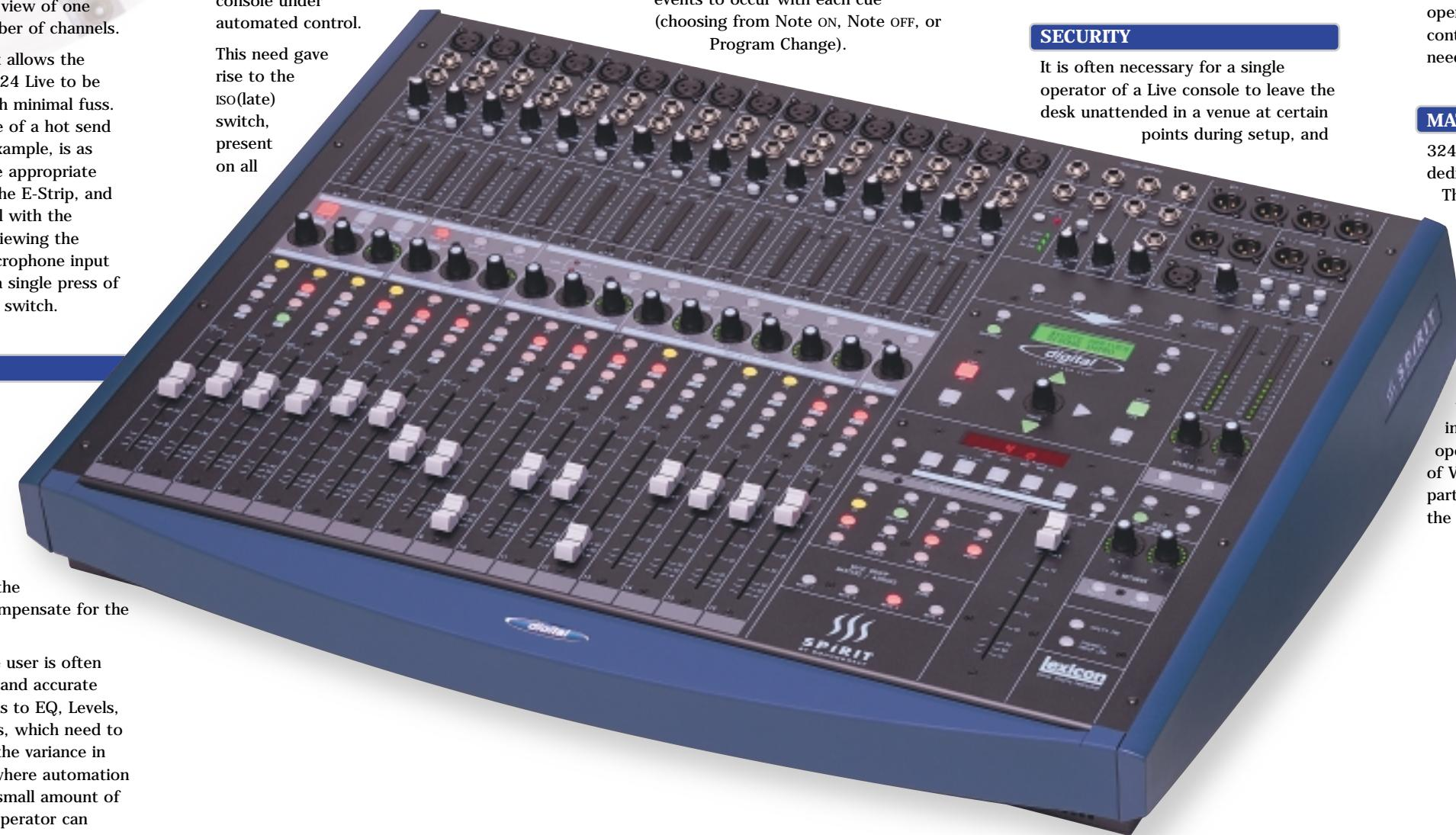
Input channels. Pressing the iso switch protects that channel from the Automation system, but still allows full manual access by the user.
