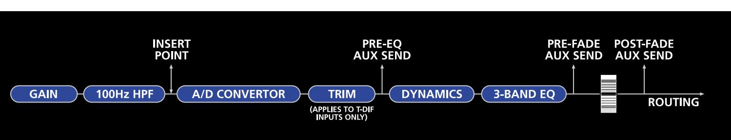
Although 324 Live is a digital mixing console, and most console functions are therefore performed in a generic DSP "block", the signal path can be shown in much the same way as that of an equivalent analogue console.
