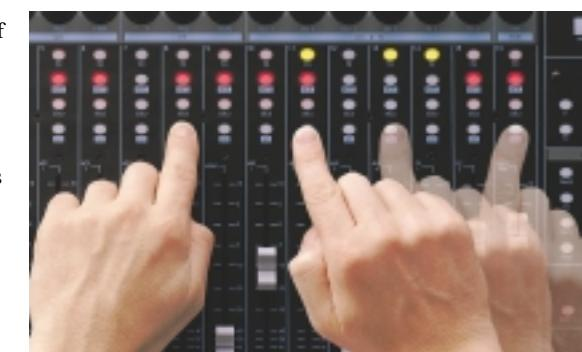
Copying of channel data is a two-button process. Pressing and holding the SELECT switch for the source channel will put the console into copy mode. At this point (still with the source SELECT held), pressing any other channel SELECT will result in the source channel data being copied across to the destination channels. Additional presses of other SELECT switches will continue to copy that information to those channels.
