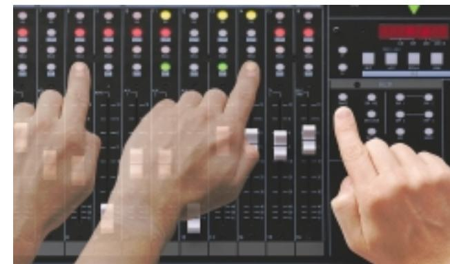
choose a switch and view the status of that switch across all channels. This feature is called "Query mode", and is activated by pressing and holding the appropriate channel switch in the SELECT panel.
