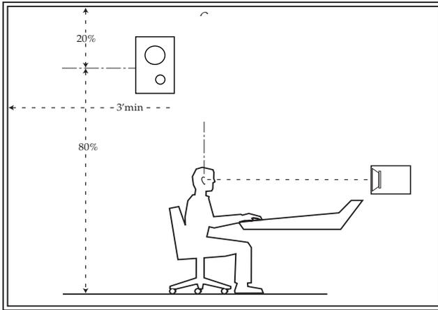
Horizontally, place the M1 Active Mk2s slightly behind the  $90^\circ$  position, at  $110^\circ$  on each side. Make sure that at the position used, there is still at least 3 feet to the back wall of your studio. If you do not have at least 3 feet to the back of your studio, then the speakers will work better if placed diagonally in the rear corner as shown on the next page.
