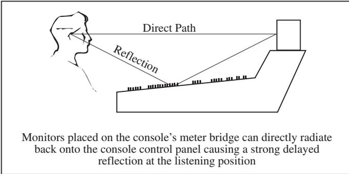
This kind of speaker placement also couples acoustic energy from the speaker's cabinet more readily into the console's chassis. Both conditions should be reduced by placing the speakers on their own stands acoustically detached from, and slightly behind, the console as shown below. In this location, the reflective path off the console's control panel is now blocked by the meter bridge.
