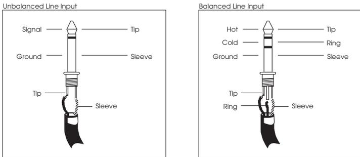
**Direct connection of unbalanced -10 dBV line level sources:** Most synthesizers, drum machines, effect devices, cassette decks and CD players operate at this level. Their average signal level is about 1/3 of a volt. They have a 2-conductor output jack that is either a 1/4" phone or "RCA phono" type. These may be plugged directly into the M1 Active Mk2's LINE IN jacks.
