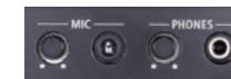
The Mic input jack on the left side panel supports plug-in power.
