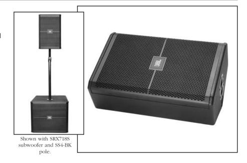
The enclosure is constructed of top quality birch plywood and coated in JBL's rugged DuraFlex™ finish. The attractive CNC-machined, 16-gauge steel grille wraps around the sides of the enclosure so there are no protruding lips on the front of the box to create acoustical interference. The grilles are internally lined with acoustically transparent foam to provide additional driver protection and give a very professional appearance.
