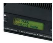
Look, no cables! A battery-powered control menu s an incredible time saver. This feature lets you configure and address the units off-site without being powered up.
