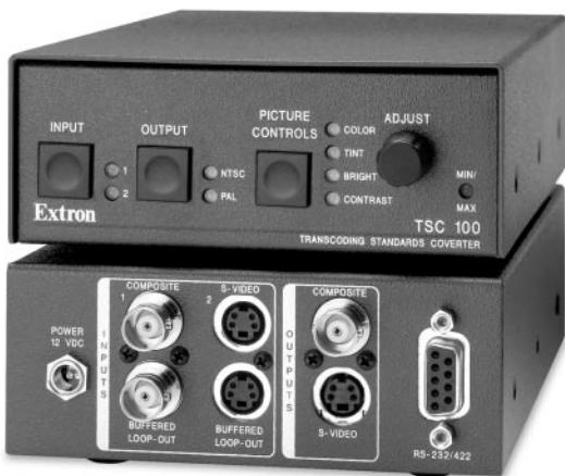
The Extron TSC 100 is a transcoder and standards converter that allows worldwide compatibility with video standards such as NTSC 3.58, NTSC 4.43, SECAM, and PAL. As a transcoder, it is able to take one video format, such as an analog composite signal, and transcode it into another video format, such as an S-video signal. It provides picture adjustment capability as well as RS-232 control.
