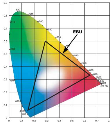
standard without resorting to colour signal processing. Furthermore, the LCD panel has a chromatic range equivalent to EBU 100%, ensuring that colour reproduction remains faithful to the original.
