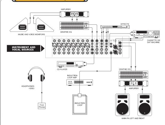
With the M Series mixer configured as shown in this diagram, it will provide a mono output to feed the main PA system, with an induction loop added for the hard of hearing. For larger scale occasions, music and voice monitor mixes may be required, which can be sent via the auxes. The main stereo mix output can also be sent to a 2-track recorder, such as a cassette or DAT recorder, if the occasion is to be recorded.
